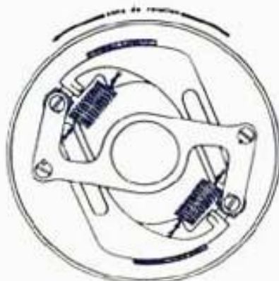
Standard clutch : view of the flyweights
