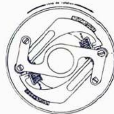
BG clutch : view of the flyweights
