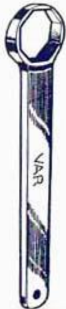
Wrench MB 1229 for upper lock screw
