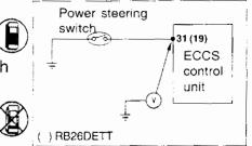
Measure the voltage between the following terminals with ECCS control unit harness connected.
