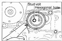
• Fix the belt tensioner and hook the spring on top of the stud volt by rotating the spring anticlockwise.
