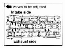
• Rotate the crankshaft one revolution (360°) and align the mark on the crankshaft pulley with the belt cover indicator. (No. 1 cylinder piston exhaust T.D.C).
