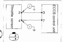
• Measure the voltage between the following terminals and ground with ECCS control unit connectors connected.
