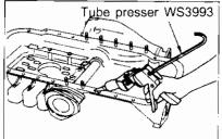
Apply liquid gasket (KP510 00150) to areas 7 mm inside from center of the oil pan bolt holes.
