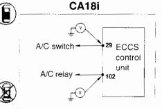
Measure the voltage between the following terminals with ECCS control unit harness connected.
