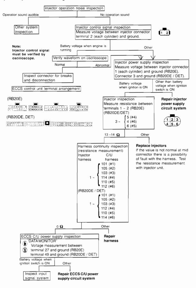
Use "POWER BALANCE" in the CONSULT active test mode to check the idle speed variation and check the injector operation.
