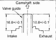
Ream inside of inserted valve guide with the valve guide ٠ reamer.
