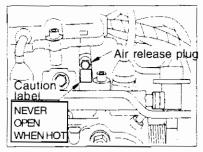
7 Stop the engine and allow it to cool. Release the radiator cap and check the fluid level. If the fluid level lowers, return to step 4 and repeat the process.
