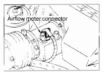
Remove airflow meter connector.
