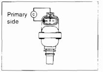
• Check the primary and secondary coil resistance value.
