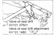
Install valve oil seal as shown.
