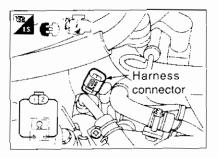
IF NG: Replace power steering hydraulic pressure switch.
