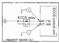
Measure the voltage between the following terminals and the ground when the ECCS control unit connectors are connected.
