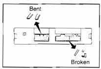
Check input / output signal before replacing ECCS C/U
