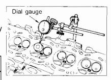
• The clearance is equal to half of the dial gauge reading.
