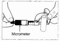
• Piston pin clearance is the figure obtained by subracting the piston pin outside diameter [Point 15] from the piston pin hole inside diameter [Point 16].
