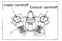
Remove the locker cover oil filler cap from intake side and check that the front end of the camshaft faces intake side.
