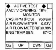
• After warming up the engine check if idle speed lowers from specified value when AAC valve connectors are removed.
