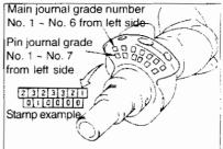
• When using undersized bearings, measure bearing inside diameter when bearing is installed and grind journal so oil clearance conforms to specified clearance.
