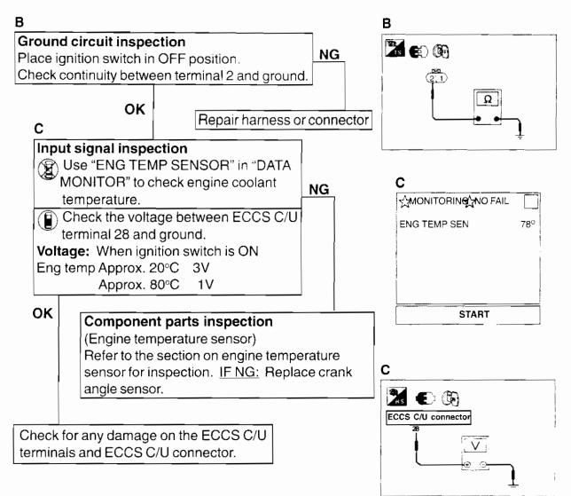
Carry out the inspection in the following order after repairs.
