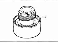
When the tensioner pulley is free, hook the tensioner spring on the upper side of the tensioner spring stud.
