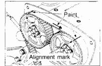
Remove the oil filter cam from intake side rocker cover and check that the front end of camshaft faces the intake side.
