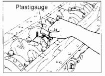
• When using undersize bearings, measure bearing inside diameter when bearing is installed. Grind pin so oil clearance conforms to specific value.
