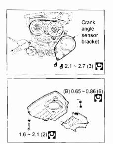
Install timing belt cover in order of lower then upper. ٠ Tightening torque (kg-m): (A) 1.6~2.1
