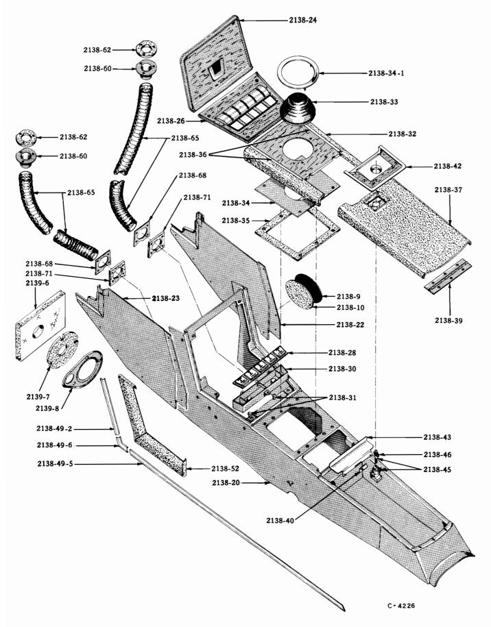
TYPICAL FRONT FLOOR BOARD AND CONSOLE (Second Design)
