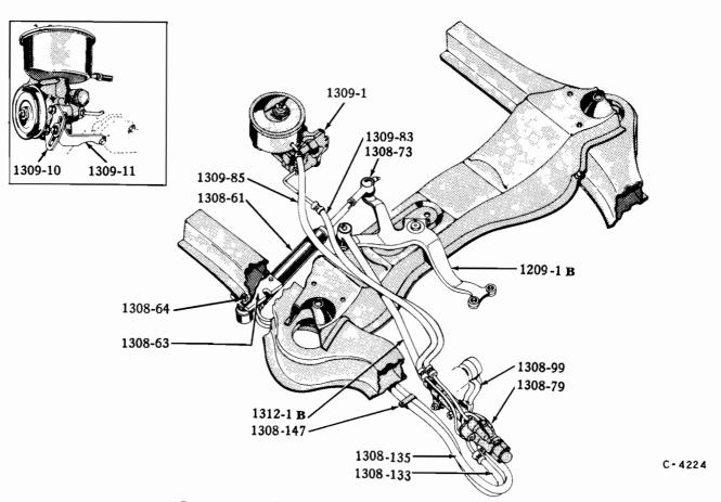
BENDIX POWER STEERING, CONTROL VALVE. POWER CYLINDER and ETC.
