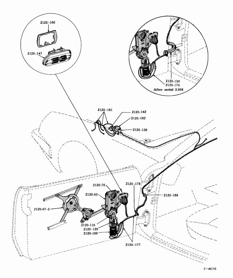
ELECTRIC WINDOW LIFT MECHANISM
